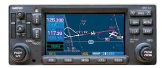
The GPS has data cards which will be kept up-to-date with the latest Garmin navigation, obstacle and terrain databases. The device will be integrated with our Garmin GTX345 ADS-B transponder which will provide Traffic alerts as well.
